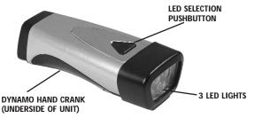
Charge the LED Flashlight by opening (flipping up) the dynamo hand-crank's handle (located on the underside of the flashlight) and hand cranking in a clockwise direction at a rate of one to two rotations per second (for optimal charging).
